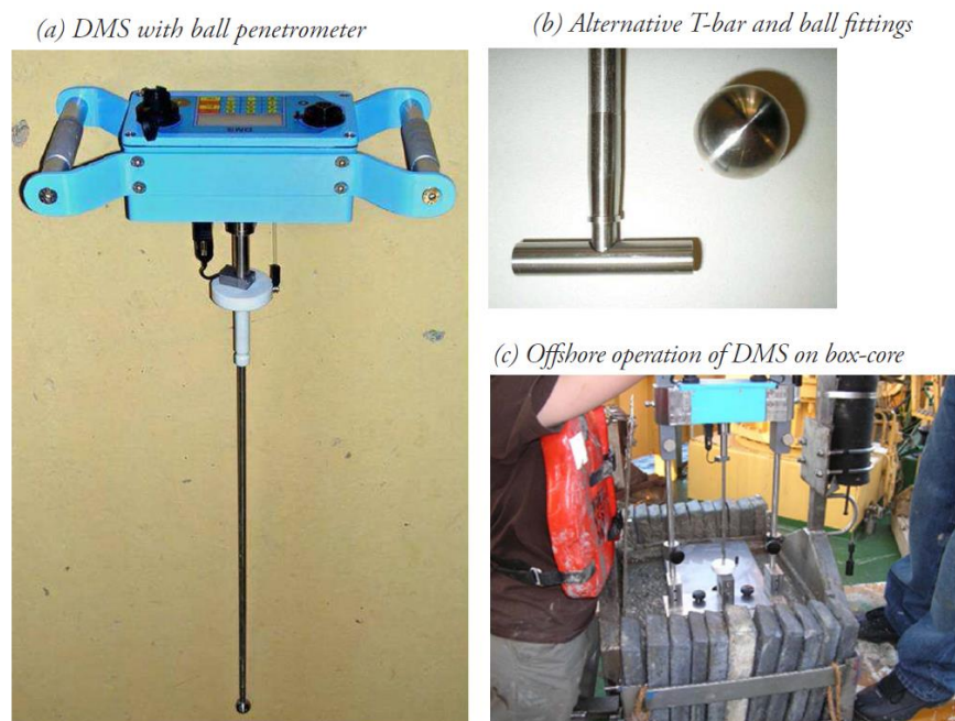
Figure 2.7 - Manually operated box-core penetrometer - the DMS (Randolph, et al., 2007)
