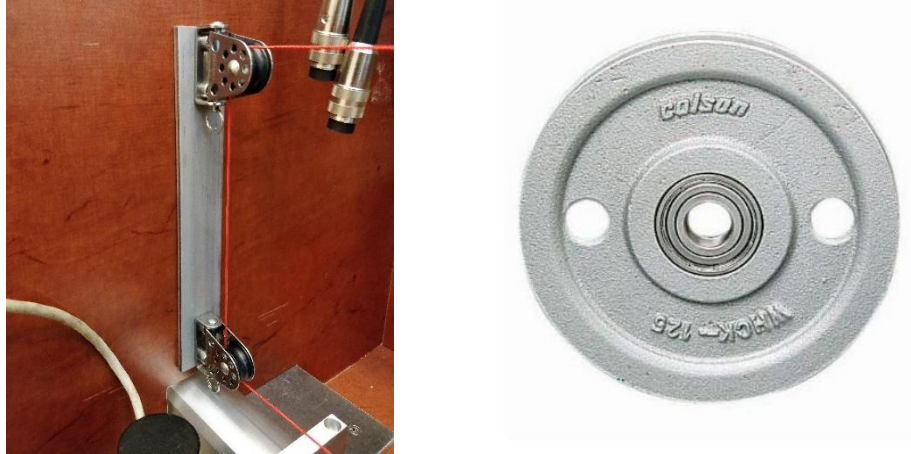
Figure 3.16- left: commercial pulleys with plastic ball bearings. Right: final pulleys with steel ball bearings
