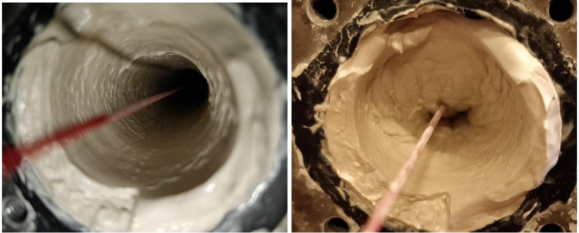
Figure 4.21 – Left: cavity created during the initial penetration. Right: cavity is closed with increasing cycles and time
