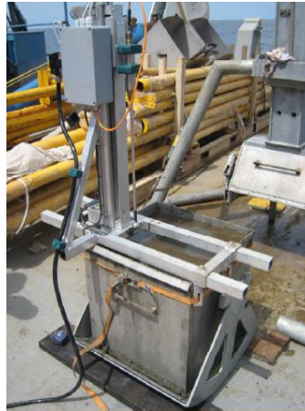
Figure 2.6 - Fugro's Deckscout mounted on a box core
