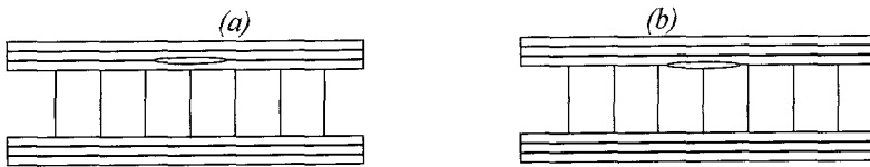
Fig. 1.1 Schematical representation of two types of delamination in a honeycomb sandwich: (a) a delamination in the skin and (b) a delamination of honeycomb material.
