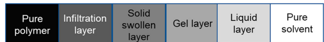
Figure 10. Schematic representation of the surface layer structure, adapted from Miller-Chou and Koenig (2003).
