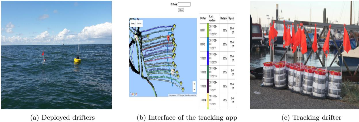
Figure 3.2: Equipment used for measuring velocities
