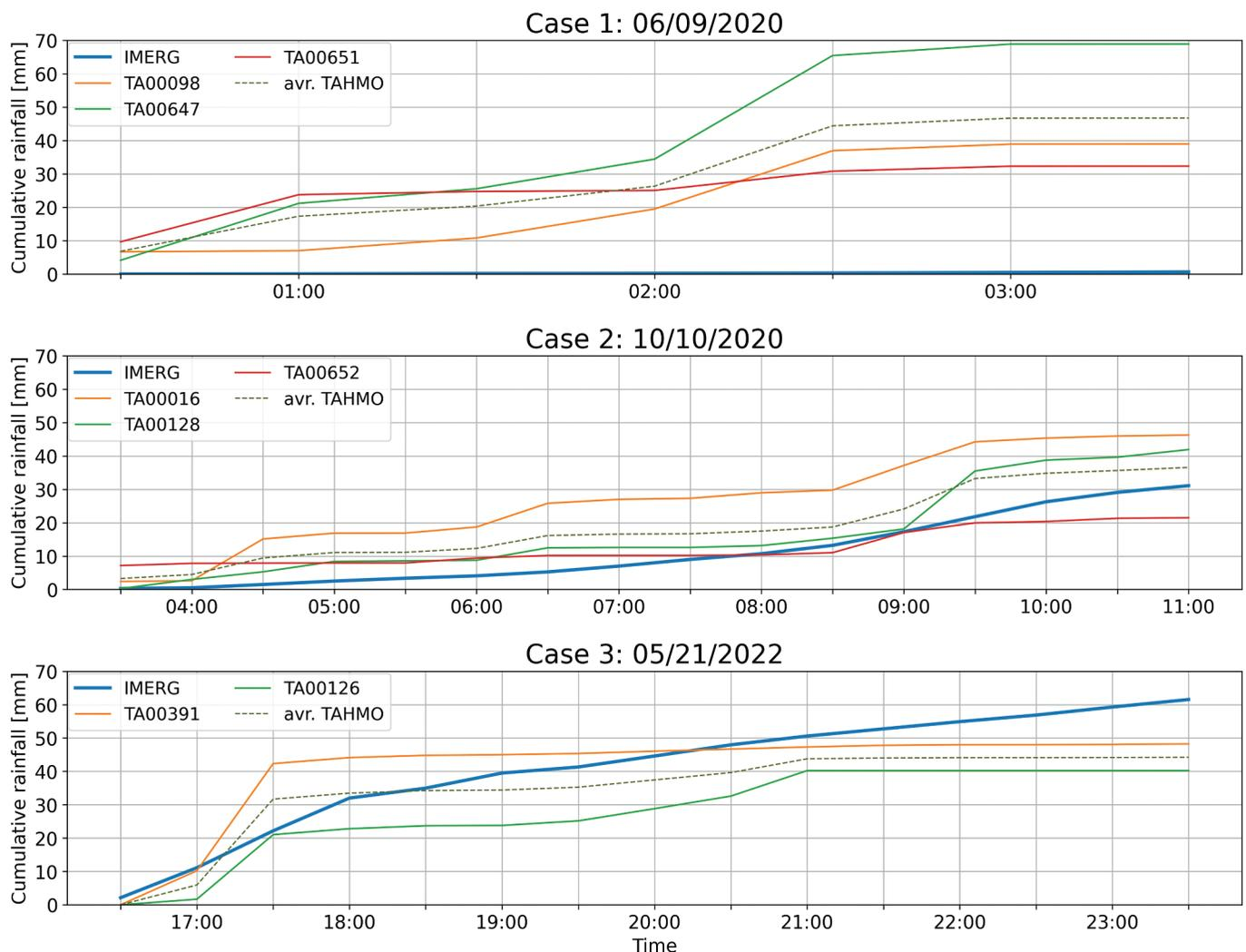
**Figure 9.** Comparison of precipitation time series from IMERG and TAHMO for the three considered events. One IMERG pixel and the various stations within that pixel are plotted for each case study. The dashed line represents the average of the selected TAHMO stations. The time interval varies per case study.
