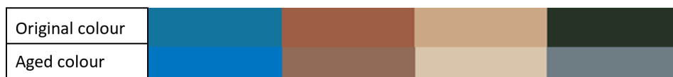
Figure 7.2: The colour change on the blue glaze layer, lips, flesh and 70/30 background paint. The original colours are at the top, the colours after the final aging step at the bottom. It can be seen that the contrast between the original colours is much greater than between the aged colours.
