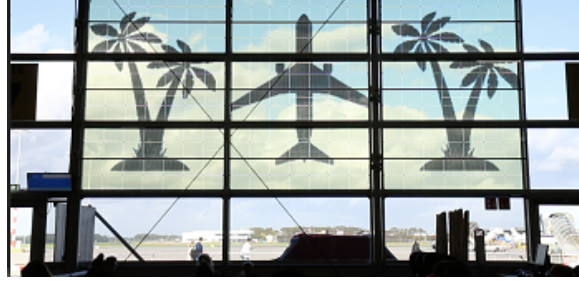
Figure 6.1: An application of passive displays: a video is shown in an airport using ambient light. The display remains transparent and does not block the outside's view. Image from [46].
