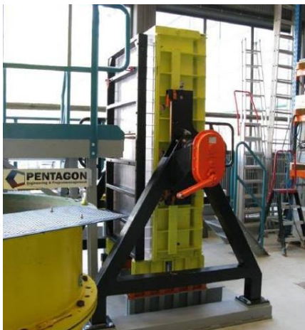
Figure D-2 a side view of the medium-scale test facility, where the box is turned 90° (Rietdijk, 2009)
