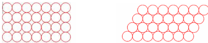
Figure 2-8 a very loose packing (left) and a very tight packing (right) (Verruijt, 2001)
