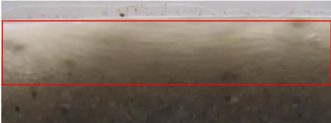
Figure 3-17 the erosion process which occurs when the channel is almost cleared Q17 03:45
