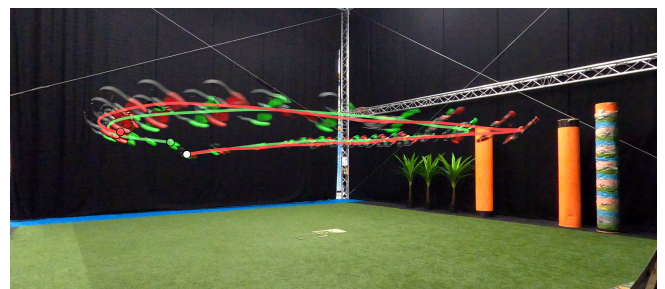
Figure 1: A comparison of a circular flight path between the proposed controller (green) and a classical PID controller (red)
