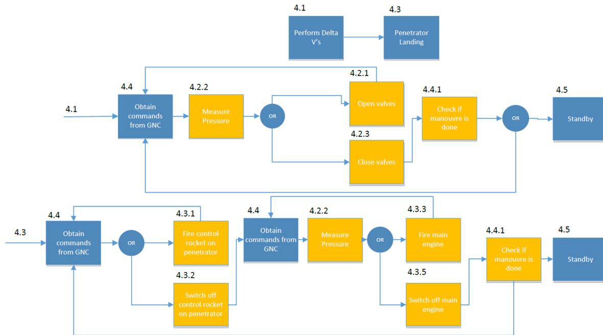
Figure 6.2: Functional Flow Block Diagram of the Propulsion System.
