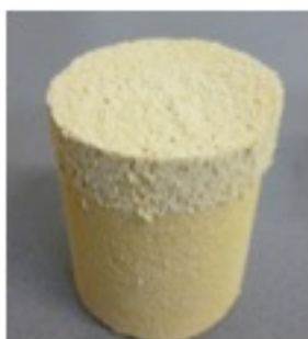
Fig. 5.1b Specimen of Maastricht limestone, with on top the re-aggregated, mortar-like layer, before treatment
