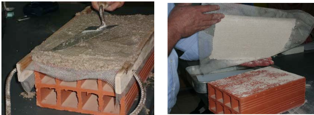
Fig. 6.2 Preparation of plaster on brick specimens for tests to be performed on the plaster: use of a glass fibre mesh (Japanese paper is also an option) between plaster and substrate and removal of the plaster after sufficient drying
