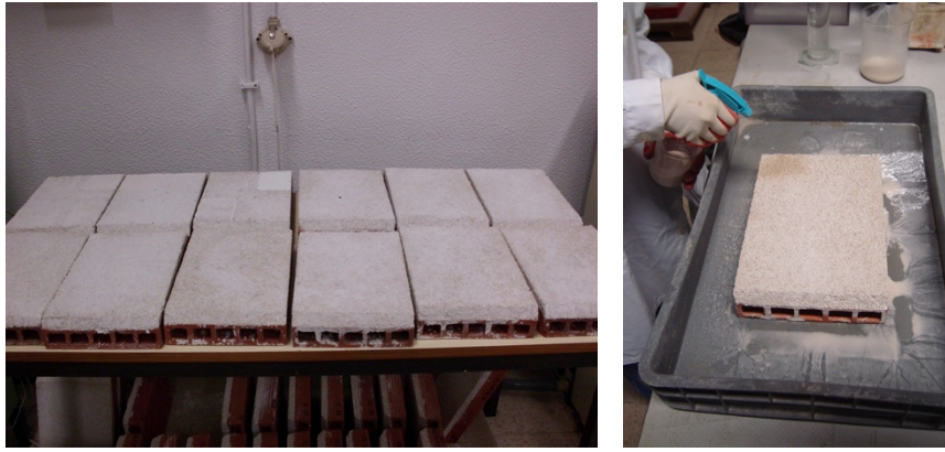
Fig. 6.1 Preparation of plaster/brick specimens and the application of a consolidant for tests to be performed on the system plaster and substrate
