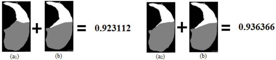
Figure 3.6: (a1, a2) Two input images (b) Ground truth; The number shows overlap value of corresponding input images with the ground truth.
