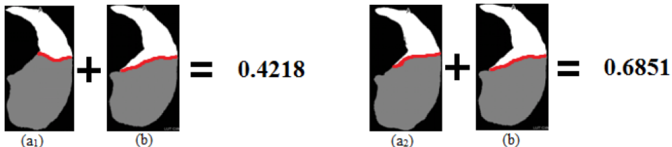
Figure 3.7: (a1, a2) Two input images (b) Ground truth; The number shows overlap value of 3 voxel wide fissures from the ground truth with that of the input images.
