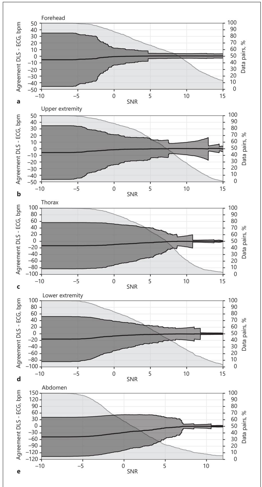
**Fig. 3.** Agreement (A-B plot) between heart rate measurements obtained with the mDLS™ sensor and ECG, plotted for every measured DLS SNR value at the forehead (a), an upper extremity (b), the thorax (c), a lower extremity (d), and the abdomen (e). Agreement is presented as bias with upper and lower limits of agreement (dark grey). The percentage of remaining data pairs (DLS-ECG) used for the Bland-Altman analyses are illustrated against the SNR (light grey).
