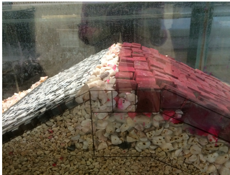
Figure 4.1: Transition from crest to rear slope filled with rock
