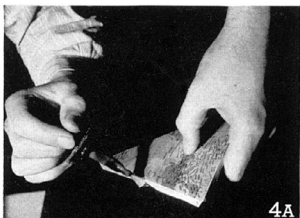
4A HOUSEHOLD PASTE or mucilage is best means for fastening flaps. It should be spread thinly to avoid warping.
