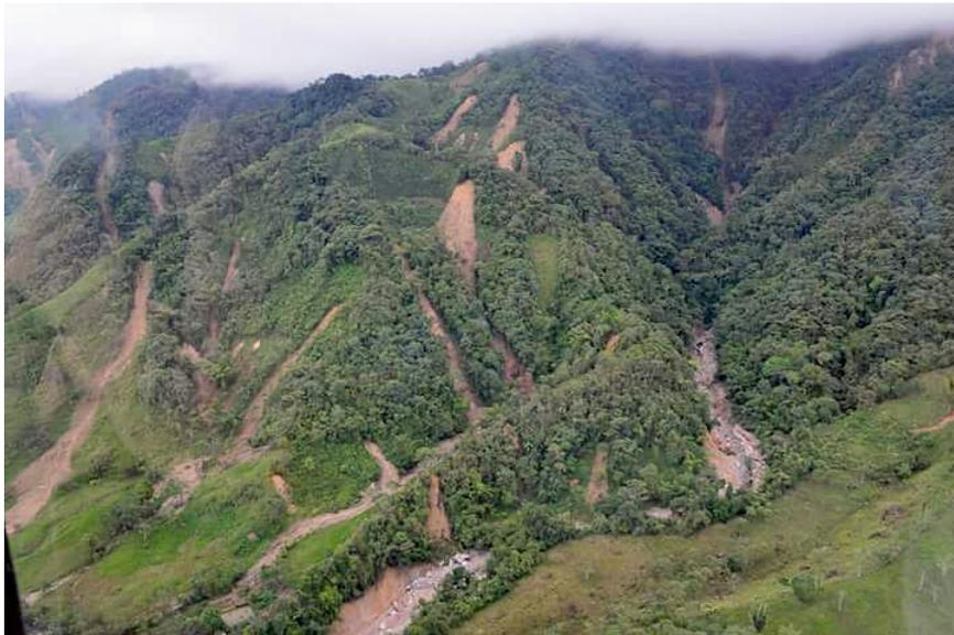
**Figure 1.23:** Multiple shallow landslides in the middle and upper part of the Taruca micro-basin courtesy Corpoamazonia via Mongabay [44].
