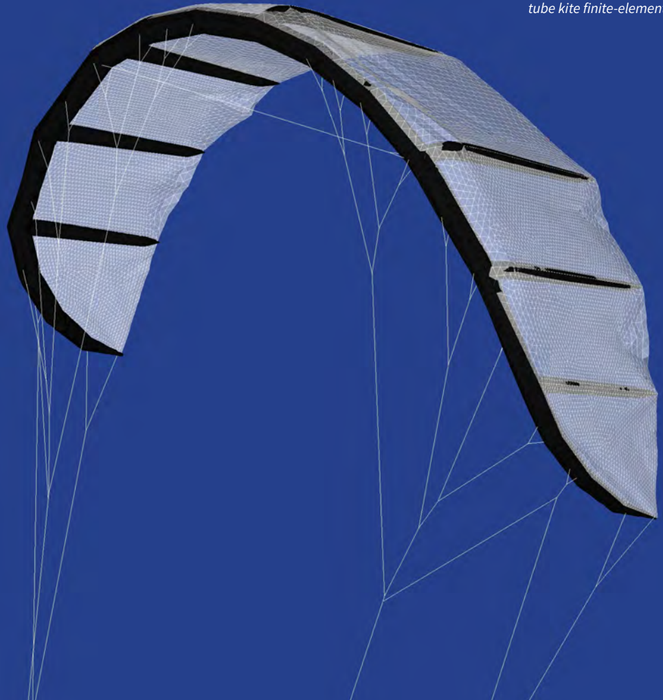
Mutiny/TU Delft V2 Leading Edge Inflatable tube kite finite-element model.
