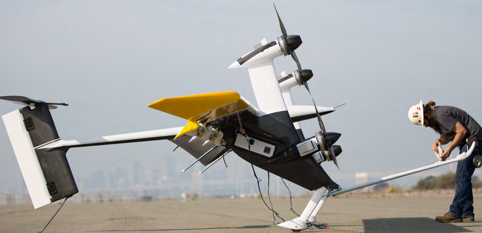
The 20 kW energy kite of Makani Power in front of the San Francisco skyline (27 November 2013).
