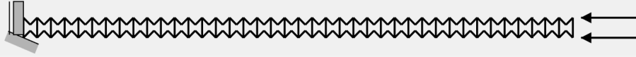
Figure 6.6: Model of re-entrant structure to estimate the longitudinal wave velocity in X1 direction
