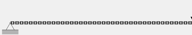
Figure 6.14: Model of re-entrant structure to estimate the shear wave velocity
