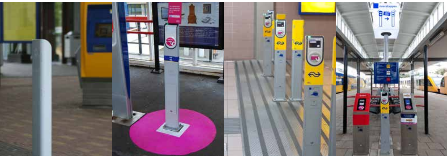
Figure 15: From left to right: No colour; with a 'cigar band' and floor markings; yellow top and in a row; transfer cube with three OV-chipkaart posts of different public transport operators.
