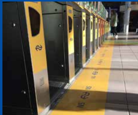
Marking for gates in a station hall: intended to indicate the distinction between public transport operators.
