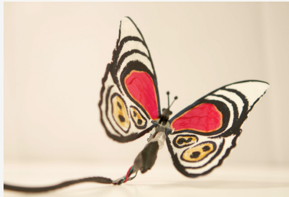
Figure 9: MoodWings: a wearable biofeedback device for real-time stress intervention (MacLean et al., 2013)
