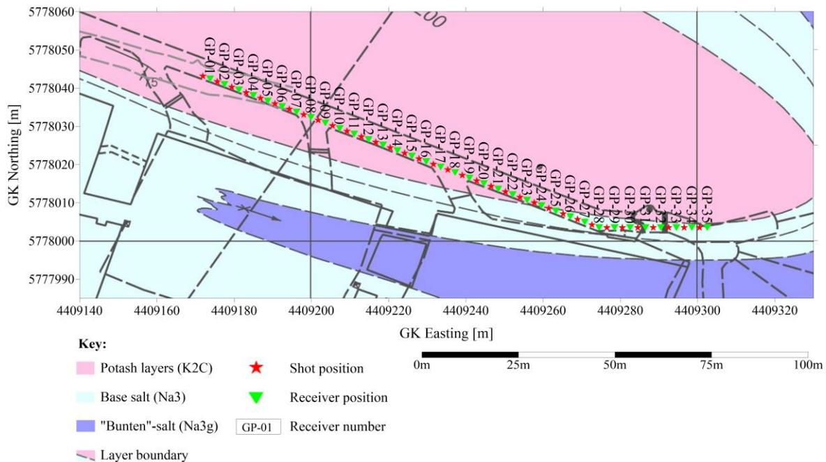
**Figure 1** Floor plan of the 574-m-deep mine gallery including the geometrical layout for the underground seismic acquisition.
