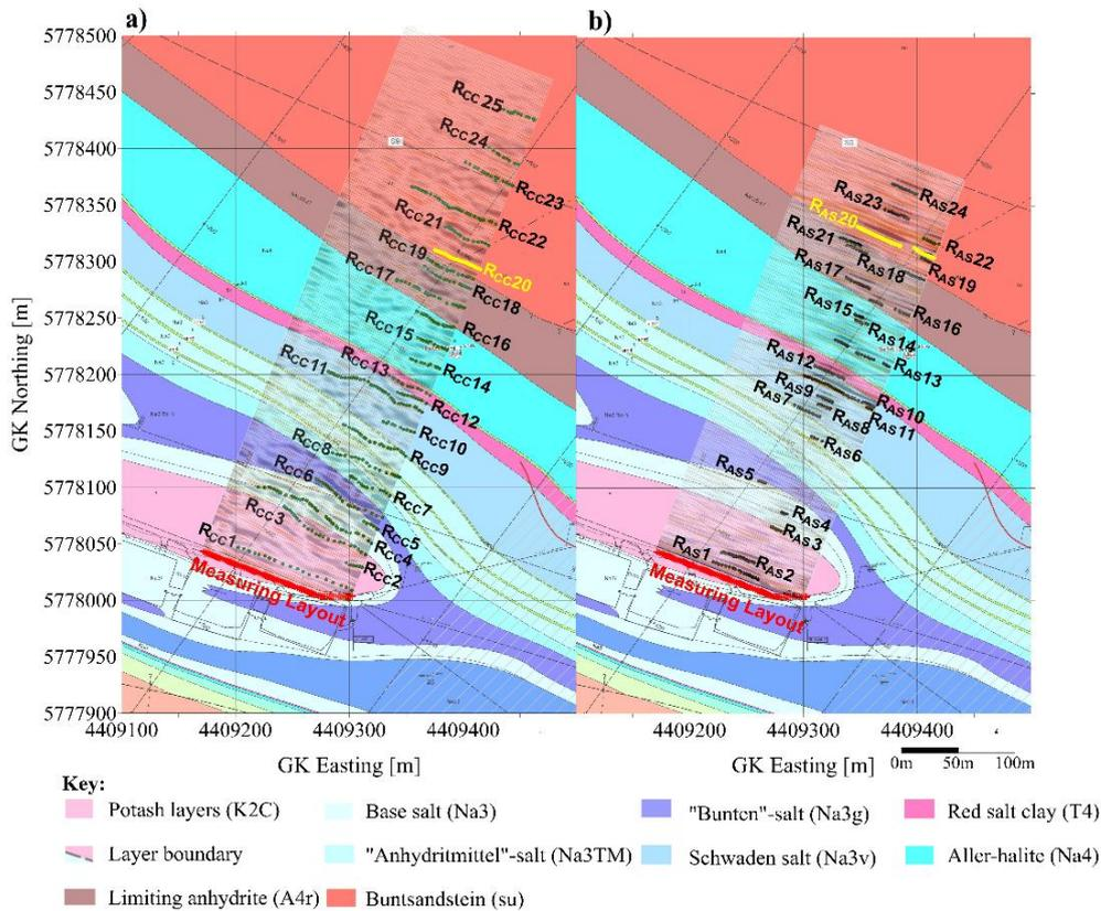
**Figure 3** Reflectors extracted from **a)**  $PSI_{-}$  (green) and **b)** the active seismic evaluation (black), projected on a 2D section of the geological model of the Asse II mine in the surrounding of the 574-m-deep gallery. The yellow reflector displays the projected limit of the salt dome.
