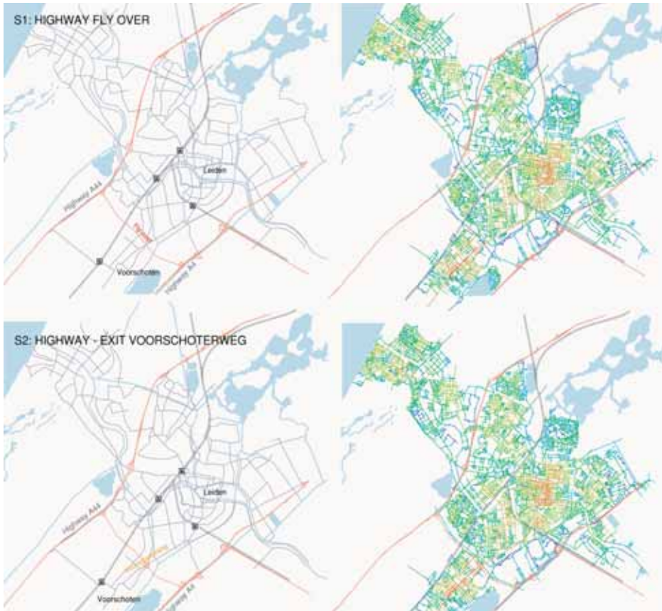
Figure 6.10 Regional-city scale networks and orthogonality analysis of two design alternatives of A11 - a. S1: Highway fly over, and b. S2: Highway with exit to Voorschoterweg.
