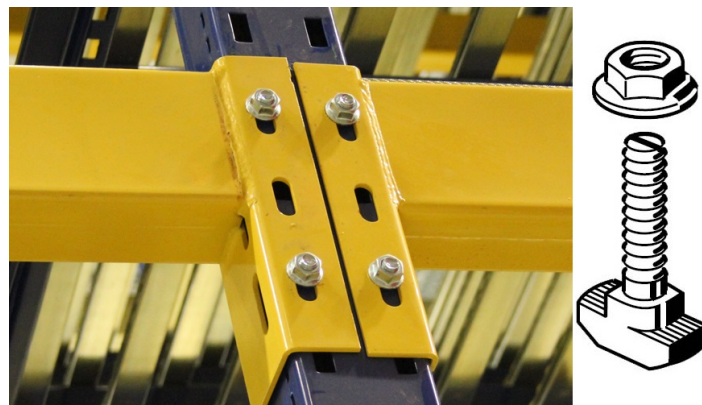
Figure 2.8: T-Bolt with limited access [13] [14]
