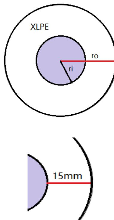
Figure2.1. Simple schematic representation of a 132kV XLPE AC cable
