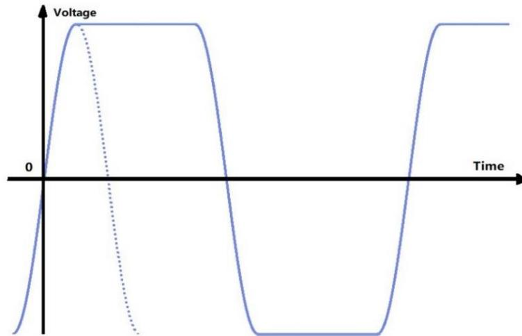
Figure 5.1 Sinusoidal in combination with DC voltage waveforms
