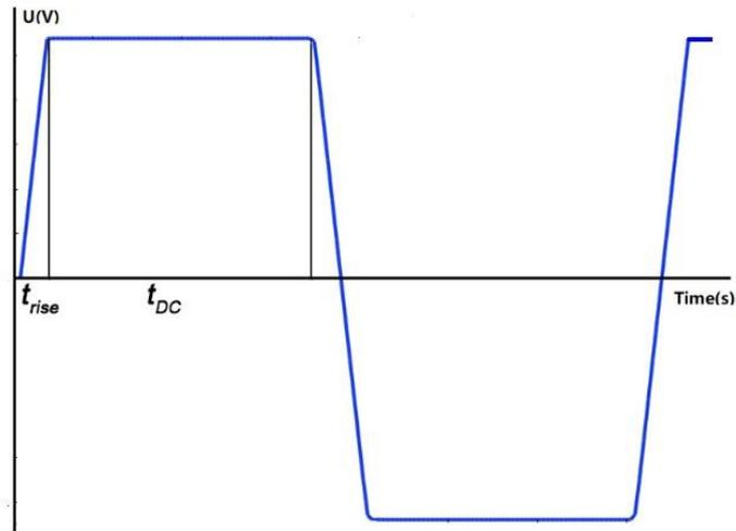
Figure 3.1 Periodical trapezoidal voltage waveform
