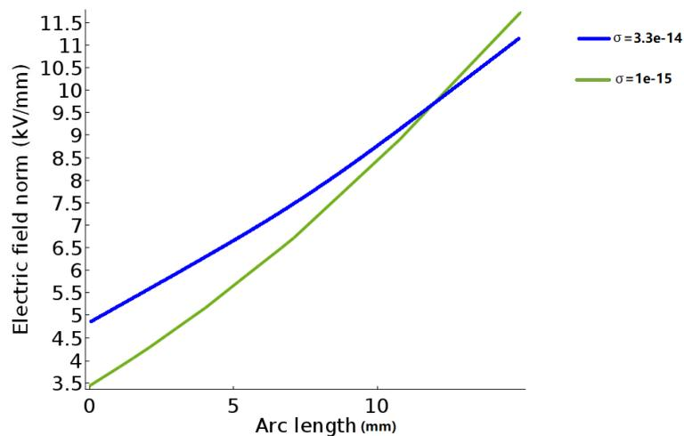
Figure6.5 Field distributions with different XLPE conductivity
