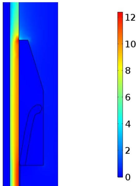
Figure7.9 Electric field at the stress cone under the optimal voltage waveform.
