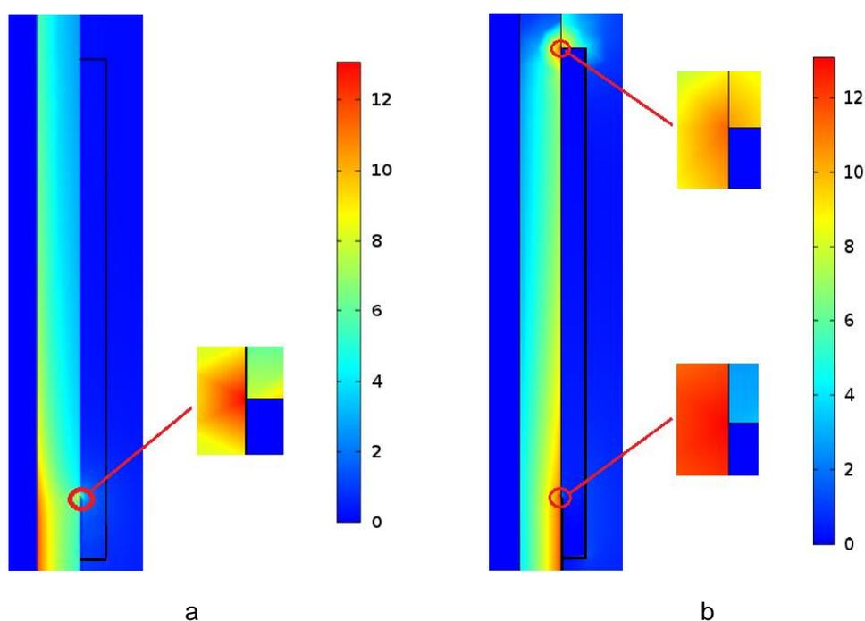
Figure 7.3 a) Electric field under AC voltage b) Electric field under DC
