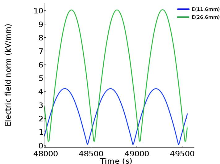
Figure2.9. Field of inner and outer points in XLPE under very low frequency AC voltage
