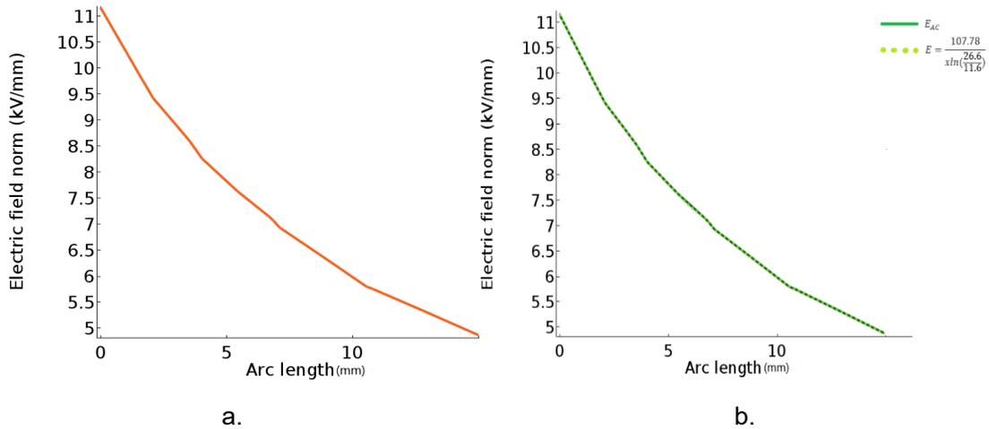
Figure2.2. a) field along XLPE arc b) E function in cable insulation with E in AC model.
