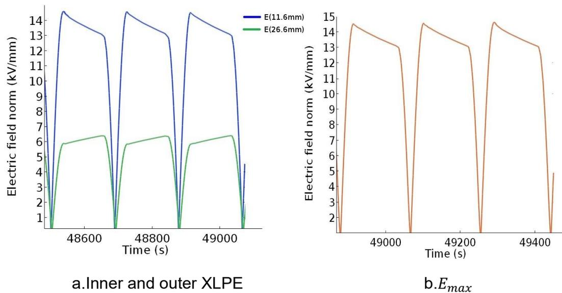
Figure 6.4  $E$  inside XLPE at 80% load current under optimal voltage waveform
