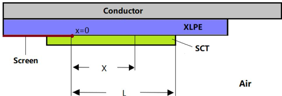
Figure7.2 XLPE cable termination with SCT field grading model
