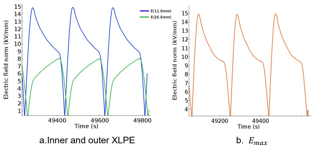
Figure 6.3  $E$  inside XLPE at 80% load current under optimal voltage waveform
