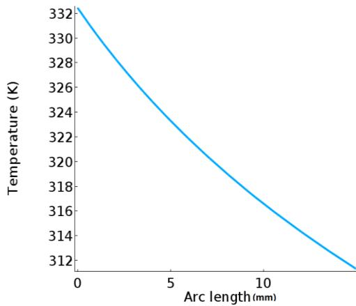
Figure2.7 Thermal gradient of XLPE
