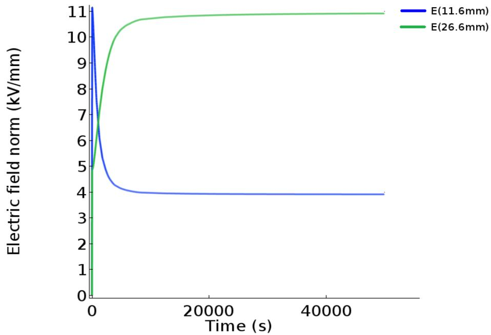
Figure2.5. Field of inner and outer points in XLPE under DC voltage
