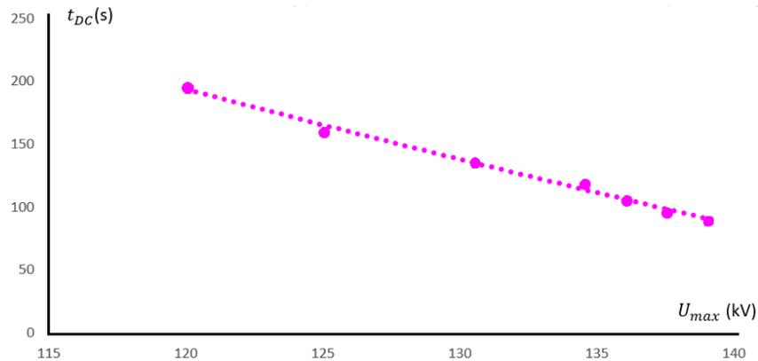
Figure4.2 Fitting curve of  $t_{DC}$  and  $U_{max}$
