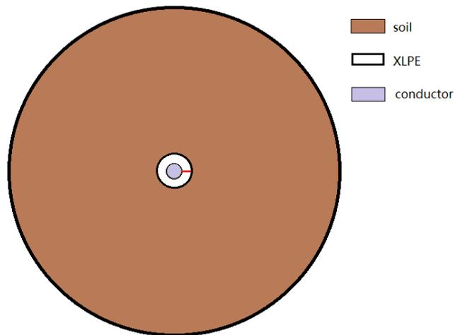
Figure2.3. An underground cable model for DC simulation.
