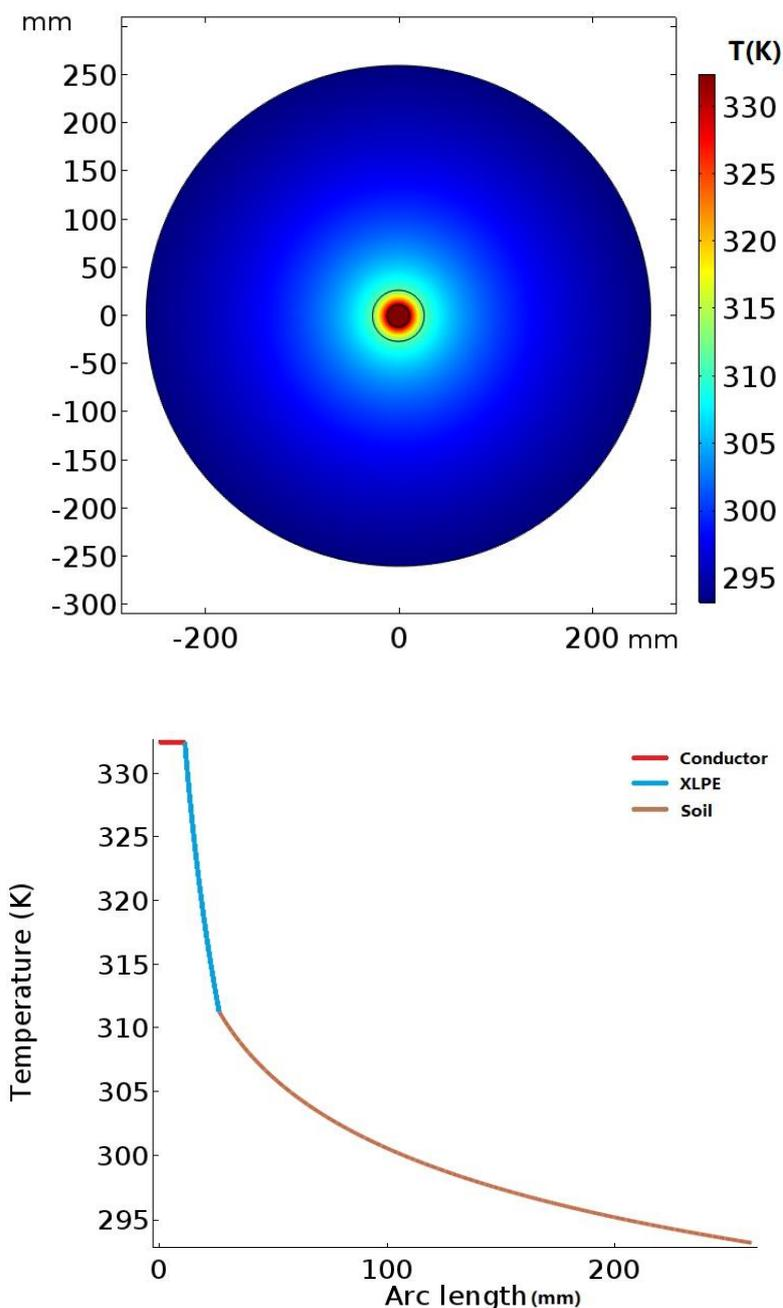
Figure 2.6 Temperature distribution at steady state
