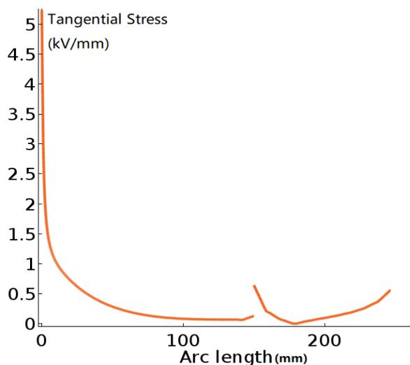
Figure7.5 Variation of  $E_{tmax}$  with x at optimal voltage
