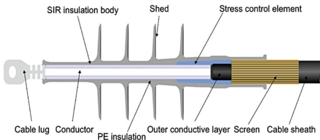
Figure7.1 A typical design of HVAC outdoor cable termination [4]
