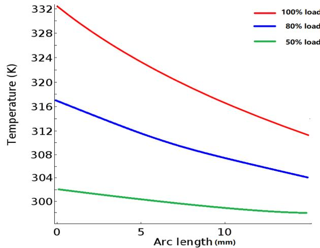
Figure6.1 Temperature gradient at different current ratings
