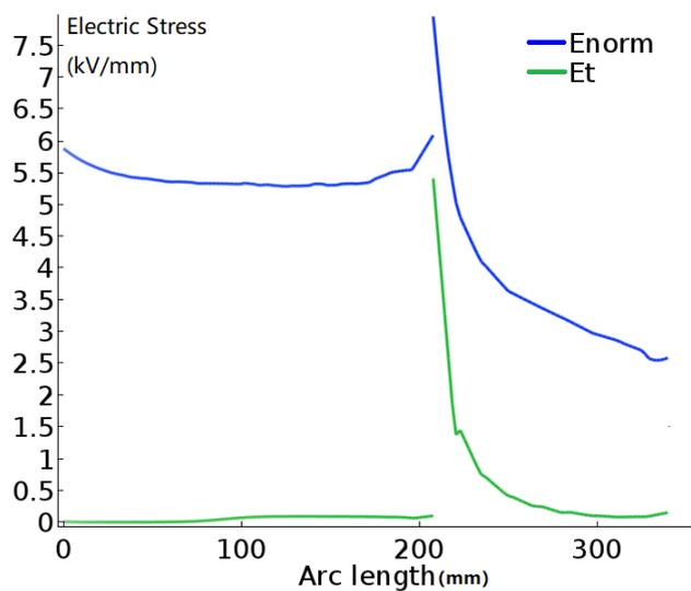
Figure7.10 Variation of  $E_{max}$  with x at optimal voltage
