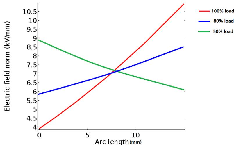
Figure6.2 Field distribution at different current ratings
