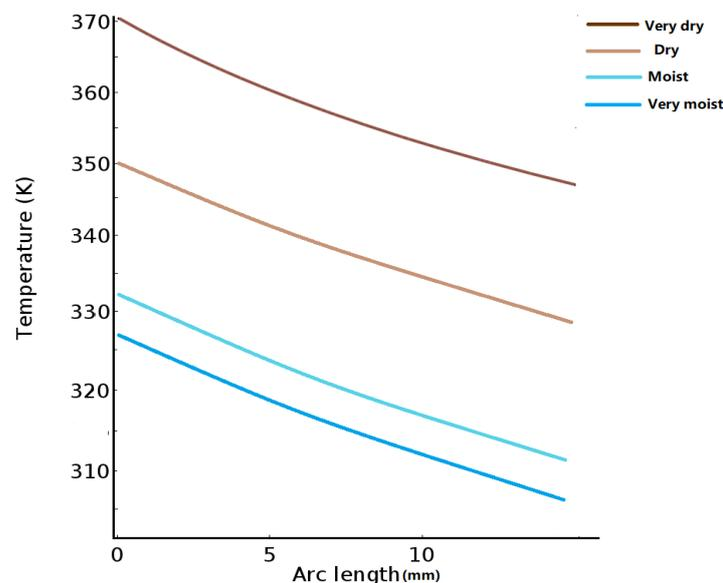
Figure6.6 Temperature distribution of XLPE surrounded by different soil conditions
