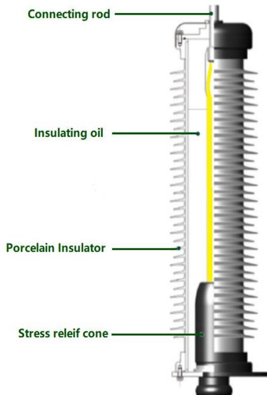
Figure7.6 Typical HVAC outdoor termination with a stress cone [10]
