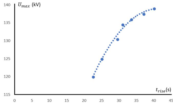
Figure4.1. Fitting curve of  $t_{rise}$  and  $U_{max}$
