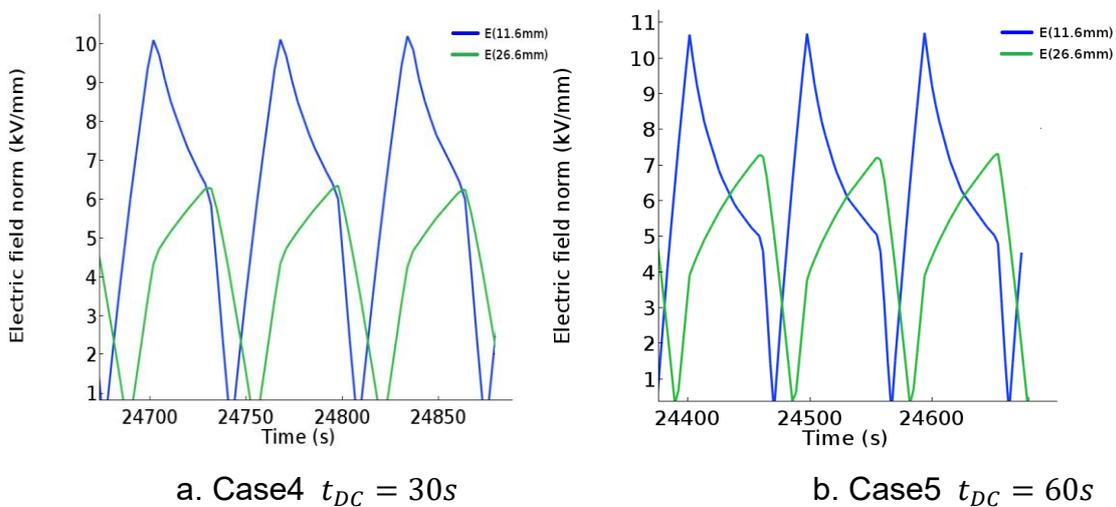
Figure3.3 Field of inner and outer XLPE under trapezoidal waveform when
