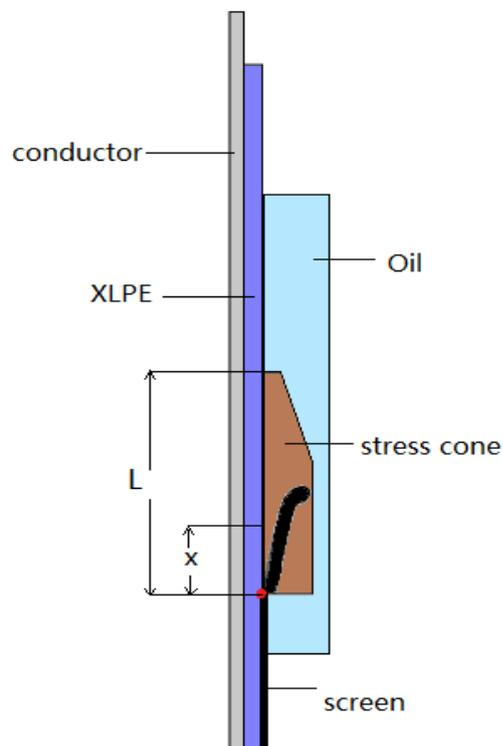
Figure7.7 132kV cable termination with stress cone model
