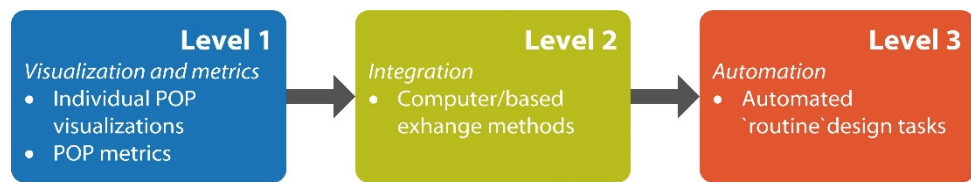
FIGURE 4.5 Schematic representation of the VDC maturity model levels (Schrama, 2011) -edited
