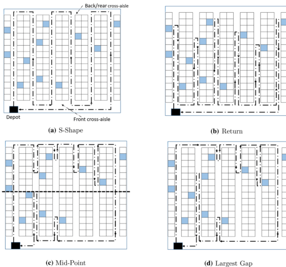
Figure 4.3: Four different heuristics used for order picker routing [59].
