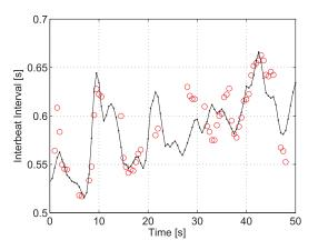
Fig. 23. Heart interbeat interval estimated using the proposed method from the output of the HPF and DCMP applied to  $s_A(t) + s_B(t)$  when there are both participants A and B. The reference ECG data (black line) and radar measurement (red circles) are shown.
