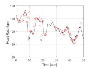
Fig. 25. Heart rate estimated from the output of the HPF and DCMP applied to  $s_{\rm B}(t)$  when there is participant B only. The reference ECG data (black line) and radar measurement (red circles) are shown.
