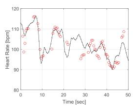
Fig. 27. Heart rate estimated using the proposed method from the output of the HPF and DCMP applied to  $s_A(t) + s_B(t)$  when there are both participants A and B. The reference ECG data (black line) and radar measurement (red circles) are shown.
