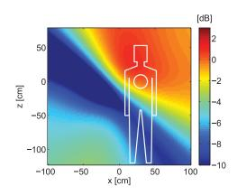
Fig. 10. DCMP antenna pattern for participant B.
