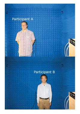
Fig. 5. Measurement scenarios with participants A and B standing in front of the antenna array.
