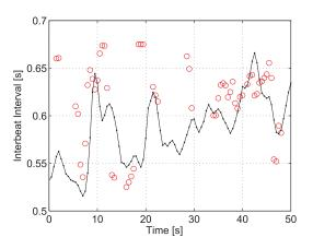
Fig. 24. Heart interbeat interval estimated from the output of the HPF and the conventional array beamforming applied to  $s_A(t) + s_B(t)$  when there are both participants A and B. The reference ECG data (black line) and radar measurement (red circles) are shown.
