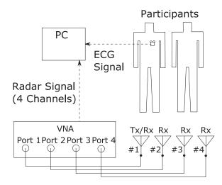
Fig. 1. Schematic of the measurement system.
