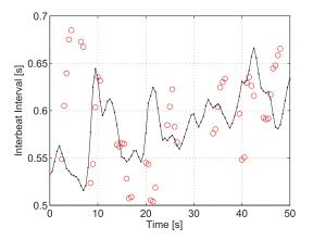
Fig. 22. Heart interbeat interval estimated from the output of the HPF applied to a single channel (ch1) of  $s_A(t) + s_B(t)$  when there are both participants A and B. The reference ECG data (black line) and radar measurement (red circles) are shown.
