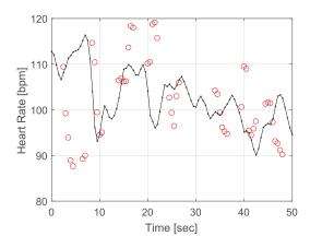
Fig. 26. Heart rate estimated from the output of the HPF applied to a single channel (ch1) of  $s_A(t) + s_B(t)$  when there are both participants A and B. The reference ECG data (black line) and radar measurement (red circles) are shown.
