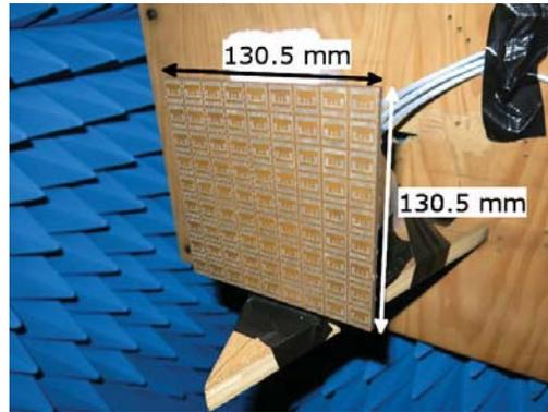
Fig. 2. Planar  $9 \times 9$  antenna array used in the present measurement.
