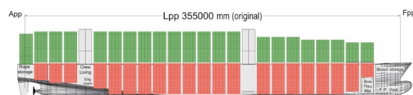
Figure 19. Potential lay-out of cargo spaces to determine container carrying capacity: 15000 TEU.
