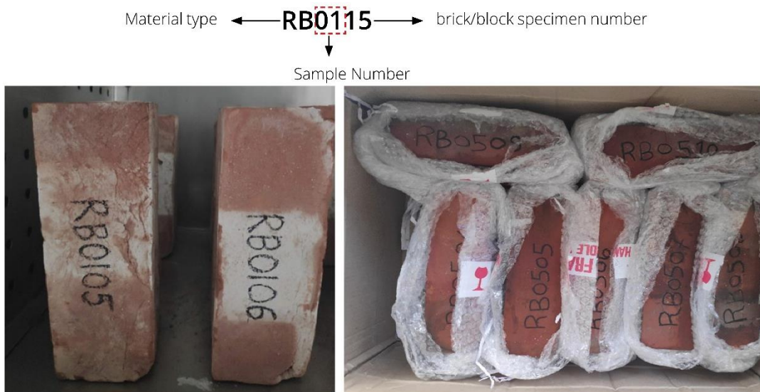
Figure 3.10: Illustration to explain sample tag(top) and photograph of tagged bricks, Rawal et al., 2020
