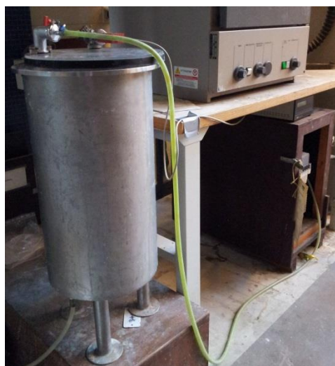
Figure 3.4 Vacuum chamber for saturation test
