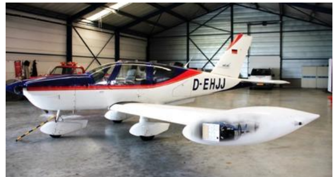
Figure 1: The test aircraft with the radar in the wingtip
