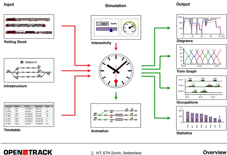
Figure 4.1: Overview of the functionalities of OpenTrack with the required input and the produced output (Huerlimann, 2013).
