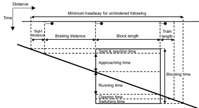
Figure 2.2: Blocking time for fixed block signalling (Goverde, 2005).
