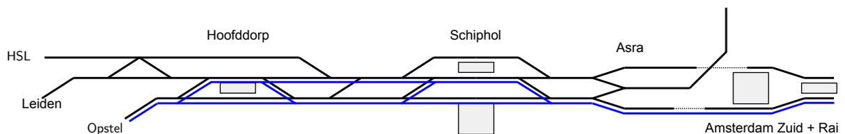
Figure 4.10: Example of rerouting possibilities for an IC train coming from the 'Zuid-as' ending at Schiphol railway station. These IC train drive further to the yard in Hoofddorp ('opstel'). In this case there are 5 possible routes.
