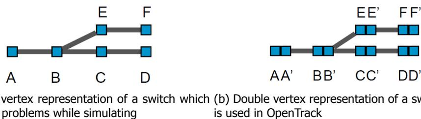
Figure 4.2: The different representations of a switch in a graph system (Huerlimann, 2003).
