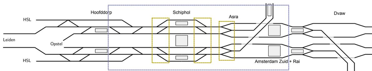
Figure 3.10: Overview of the 2018 Schiphol railway network. The large, blue area shows the control area of the DVM system. The smaller, orange areas show the steering areas.
