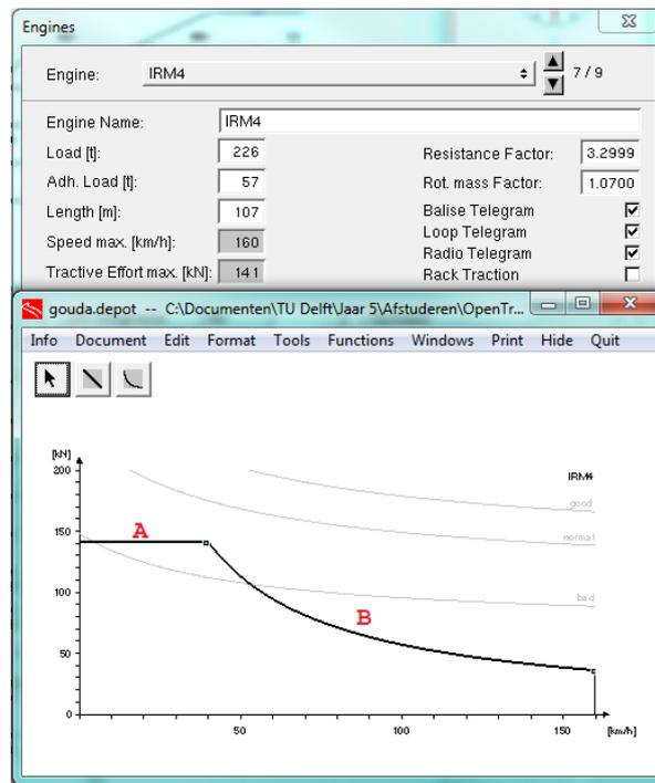
Figure 4.4: Example of what the rolling stock data looks like in OpenTrack, with the entry fields of the basic data and the traction-force curve. A is the traction-force limited due to adhesion, and B is limited by the engine power. (OpenTrack).
