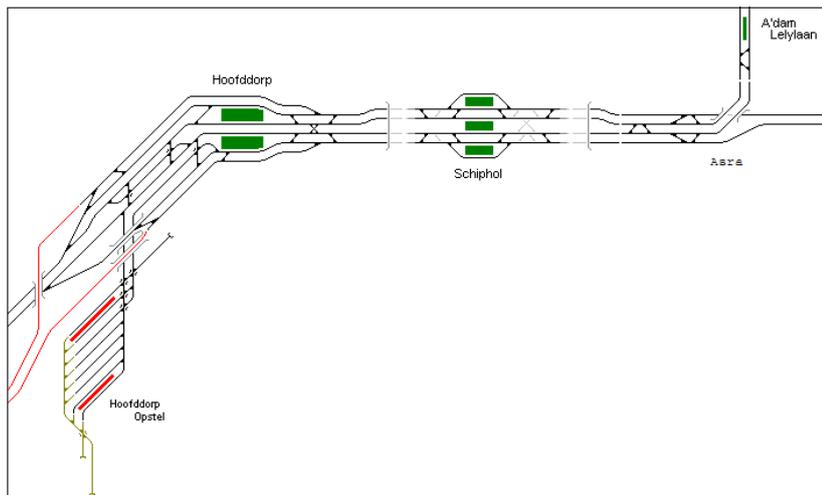
Figure 1.2: Topology of the Schiphol area (sporenplan.nl).
