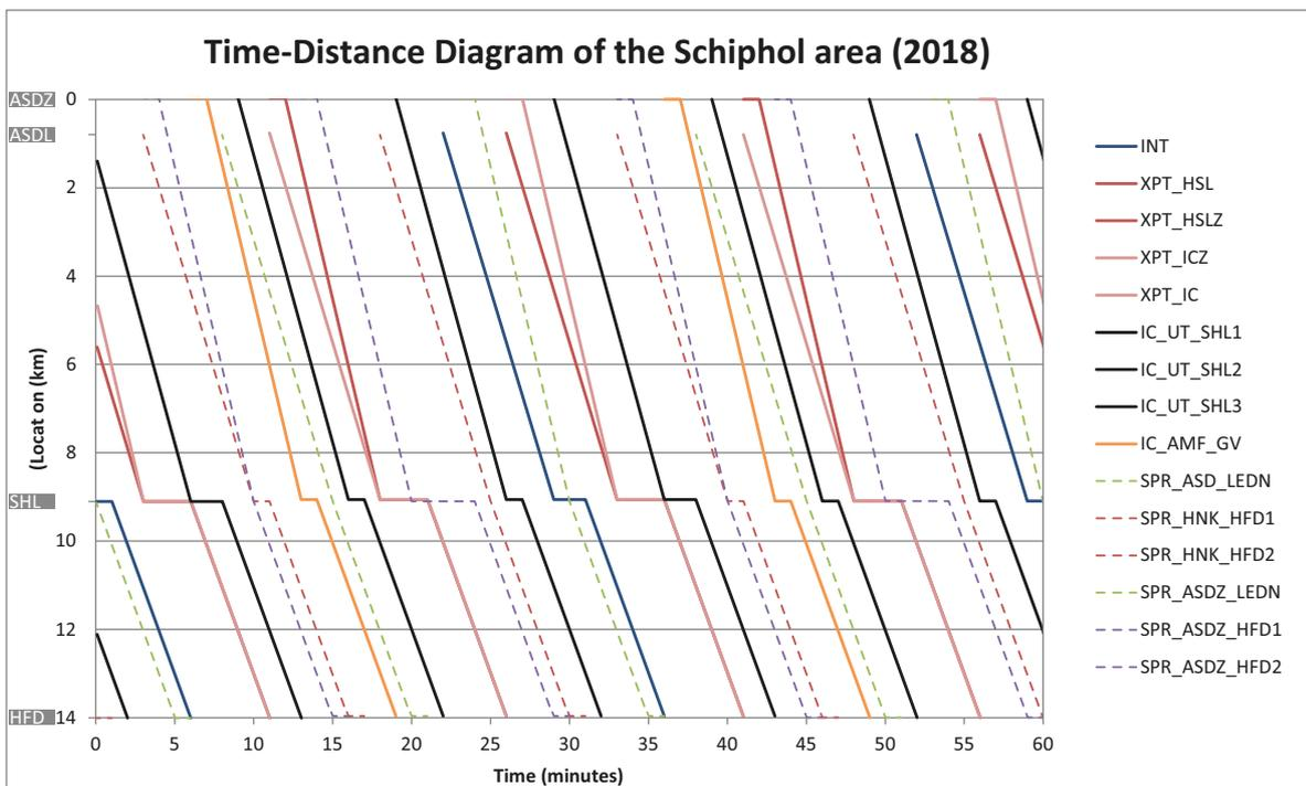
Figure 4.5: Possible timetable for the future situation including the XPT. The abbreviations of the train series are explained below in table 4.2. The timetable is showed in the form of a time distance diagram where the branch from Amsterdam Zuid and Amsterdam Lelylaan are plotted on top of each other.
