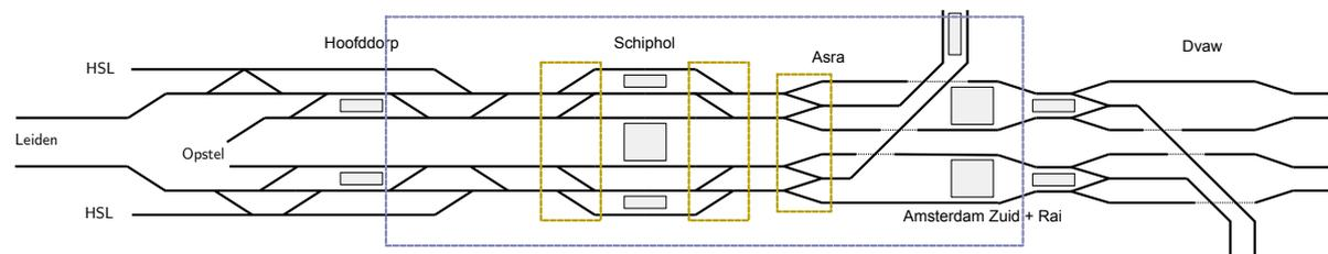
Figure 2: Overview of the 2018 Schiphol railway network. The large, blue area shows the control area of the DVM system. The smaller, orange areas show the steering areas.
