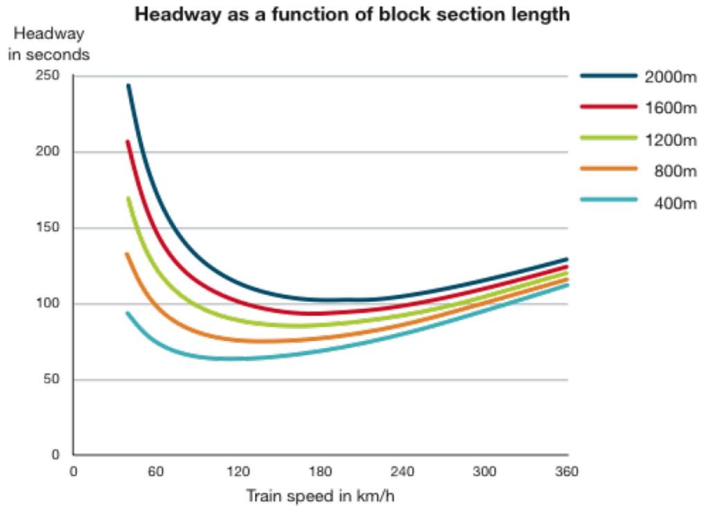
Figure 2.6: The minimum headway as function of the maximum speed and the block length using ERTMS level 2 (Hunyadi, 2011).
