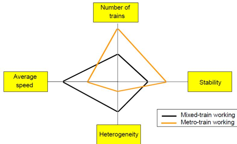
Figure 2.5: The utilisation balance. The heterogeneous model in black, the corridor or metro model in orange (Schaafsma, 2001; UIC, 2004).
