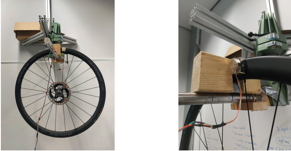
Figure 3.3: On the left, an image of the experimental set-up can be seen. The rim is freely suspended in a wooden block to prevent motion in other directions than the cycling direction. The angular speed sensor is attached close to the rotation point, on the rim. On the right, a close up of the sensor and the wooden block can be seen.
