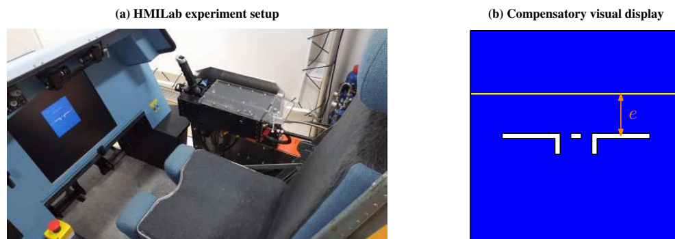
Figure 6. The fixed-base flight simulator of the TU Delft Human-Machine Interaction Laboratory (HMILab) (a) and the compensatory display (b) used for the experiment.
