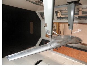
(b) ZEFT model without winglets
