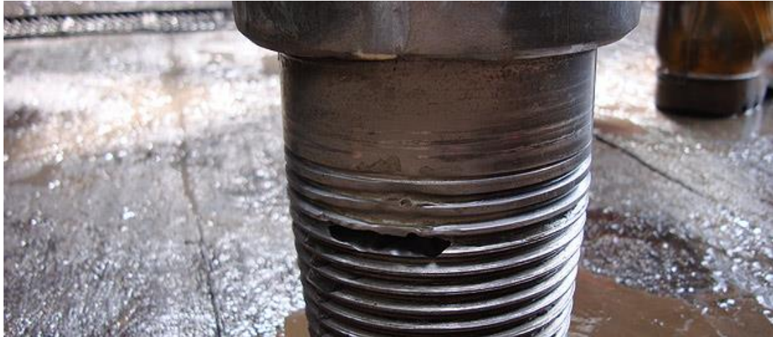
Figure 6.12: Wear of the pin connection of a drill pipe.
