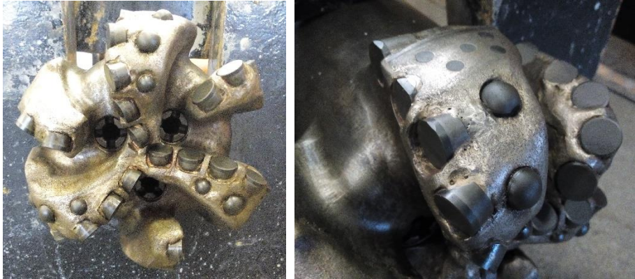
Figure 2.5: The matrix body structure (left) and the PDC cutting elements (right).
