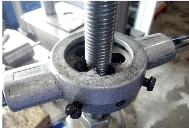
Figure 5.9: Tapping tool to repair the damaged thread.
