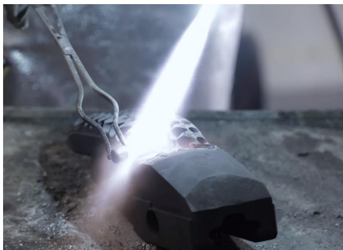
Figure 5.44: Brazing PDC bits onto the cutter block of the UR.
