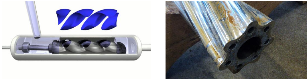
Figure 2.8: Mud motor principle (left) and rotor (right).
