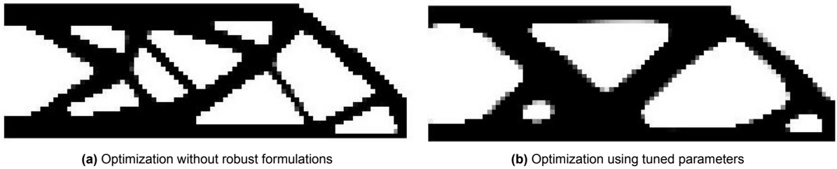
Figure 2.5: Effect of the robust formulations on the design
