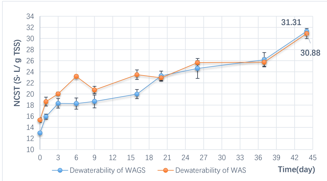
Figure 14. Different dewaterability deterioration during anaerobic digestion for WAGS and AS.
