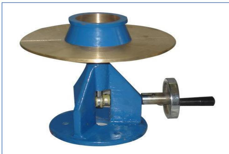
Figure 3.5 A typical slump test tool for mortars (© Accro-tech Scientific Industries., 2019)
