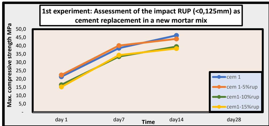
Figure 4.2 The diagram of the compressive strength test of the 1st experiment
