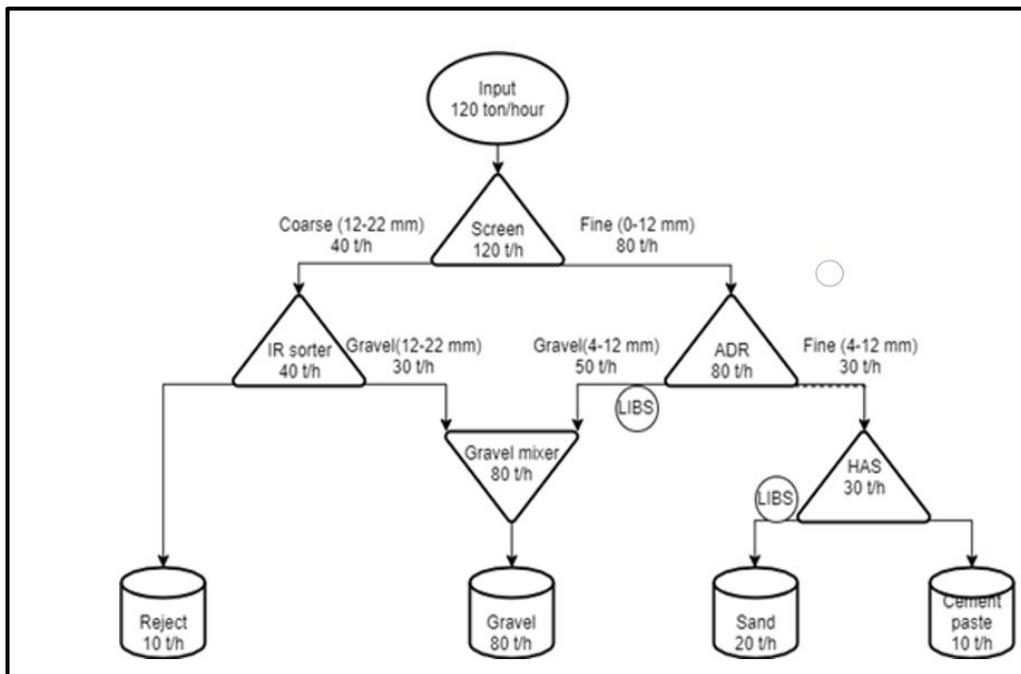
Figure 5.1 A scheme of an innovative conceptual recycling plant with usage of HAS
