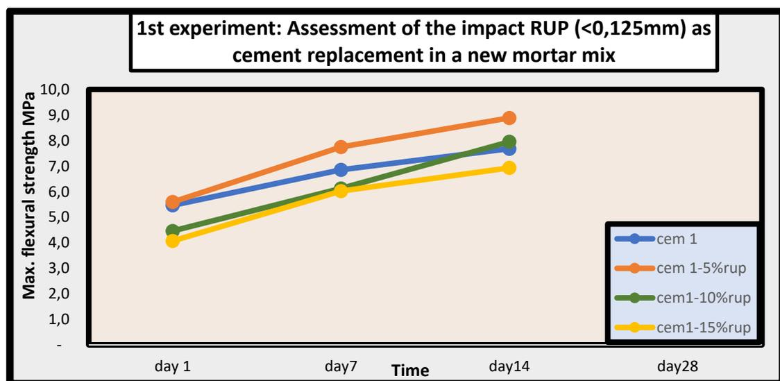
Figure 4.1 Diagram of the flexural strength test of the 1st experiment
