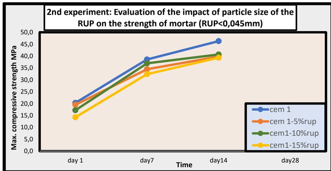
Figure 4.4 The diagram of the compressive strength test of the 2nd experiment
