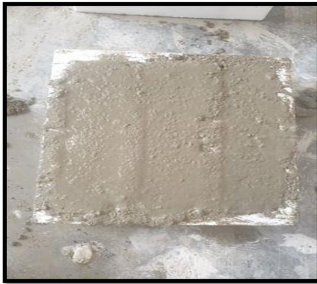
*Figure 3.6 The fresh mortars in the jolting table in the concrete lab of TU DELFT*
