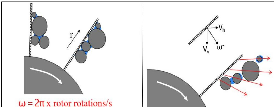
Figure 2.2 Closeup of the grain-motor interface (Bakker, 2014)
