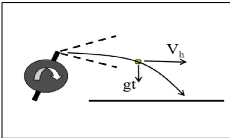
Figure 2.3 Dynamics of the ADR motor projectile (Bakker, 2014)
