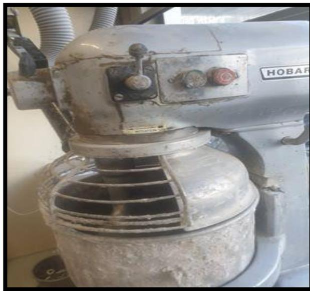
*Figure 3.3 The mixing machine and the bowl in the concrete lab of TU DELFT*
