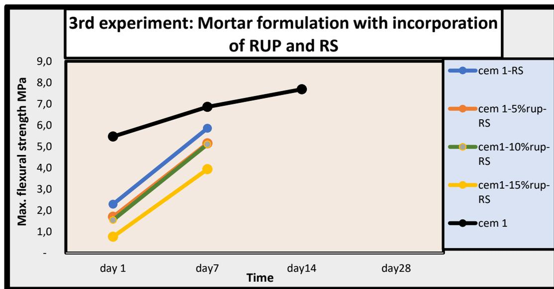
Figure 4.5 The diagram of the flexural strength test of the 3<sup>rd</sup> experiment
