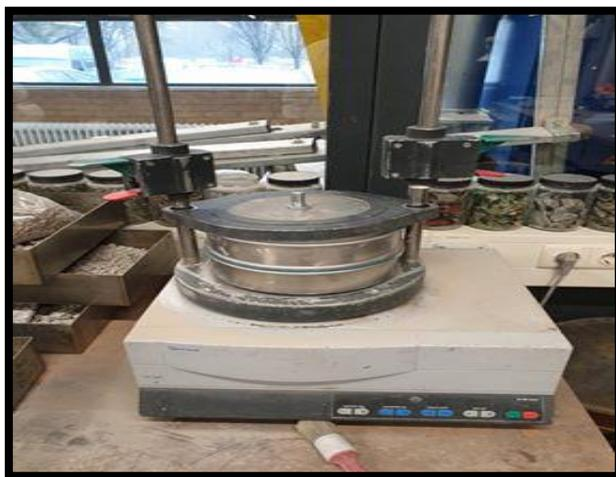
Figure 3.9 The sieving machine during 2<sup>nd</sup> experiment in the concrete lab of TU DELFT
