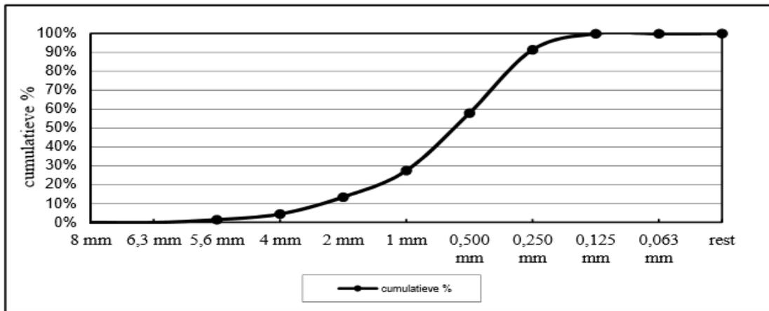
Figure 3.1 The cumulative percentage of size distribution of natural sand (DELFT\_Concrete\_Lab, 2020)
