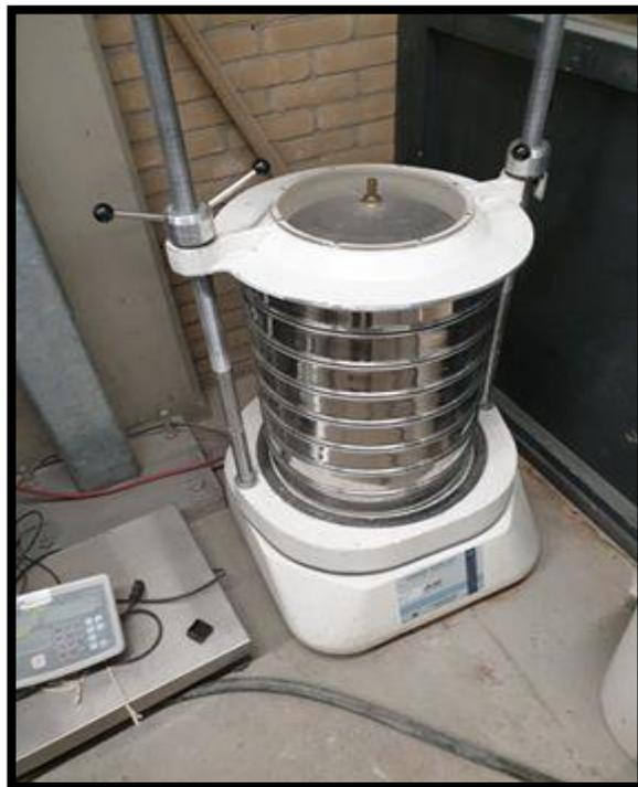
Figure 3.10 The sieving machine during 3<sup>rd</sup> experiment in the concrete lab of TU DELFT
