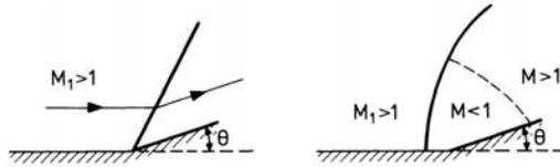
Figure D.16 Supersonic flow in a corner
