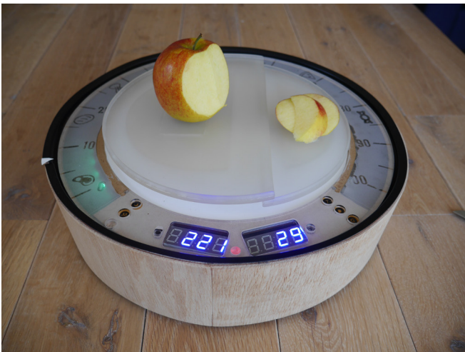
Fig. 41: Pictures showing the different functions of the working prototype: top-left: entering the carb ratio using the outer ring, top-right: Placing a product on the food plate, bottom-left: dividing the apple until the lights blink green, bottom-right: Adding up all ingredients to read the total sums
