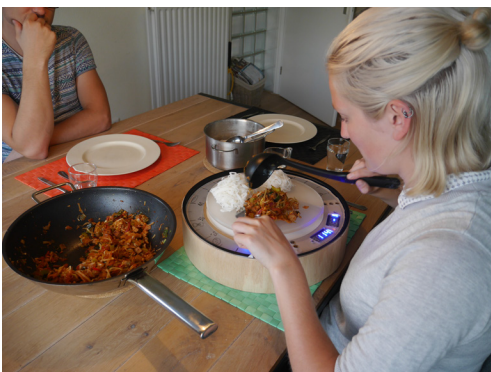
13. Again the ingredient (mixed meal in this case) can be redivided over the plates until the light starts to blink green.
