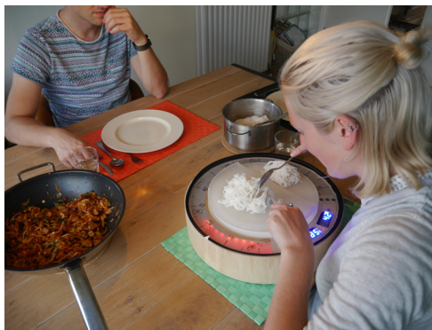
8. The color of the light indicates whether the estimation is made correctly or not. Red means wrong and green means correct.
