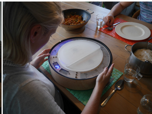
5. When being turned on the lights on the scale start to go round. First, the carb ratio for the first ingredient has to be entered by turning the outer ring.
