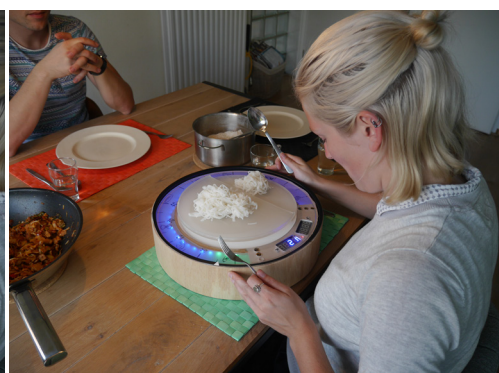
11. Now the ring can be turned to the ratio of the next ingredient. The color of the ring will return to blue and the screens grams will go back to 0.
