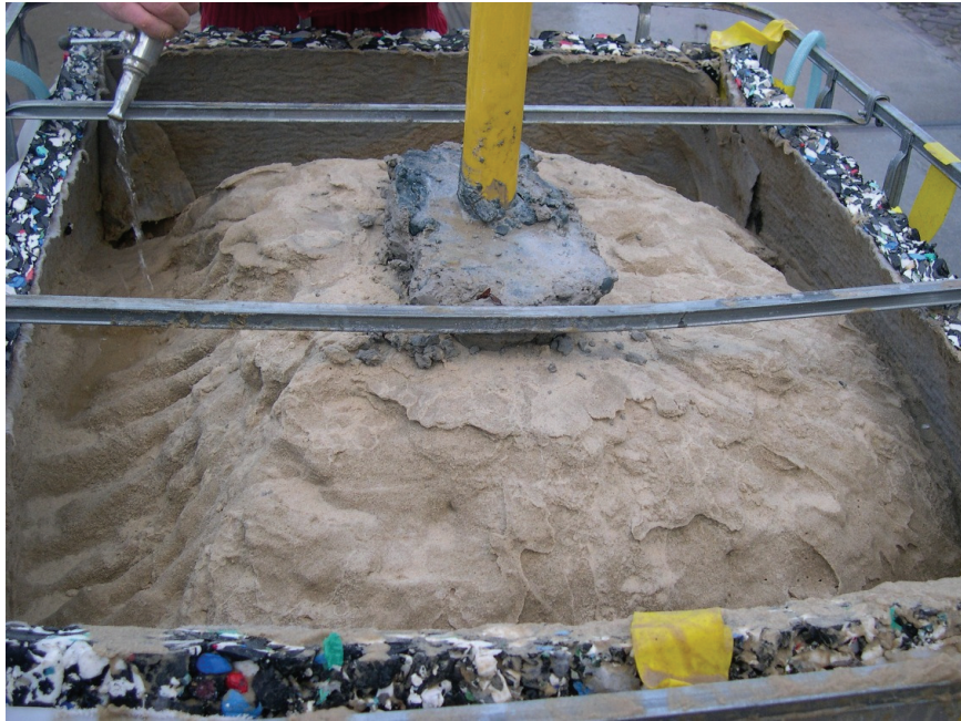
Figure 2 The surface of the cemented sand body of the second cubic meter test. Ridges with high \text{CaCO}_3 content are visible in a regular patterns on the left.
