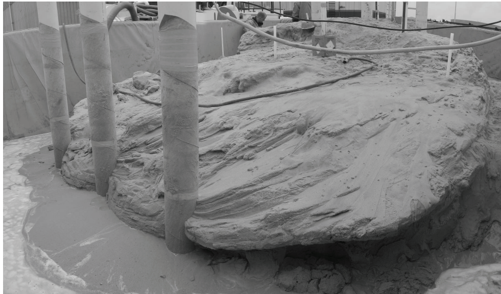
Figure 2 Cemented sand body observed from the corner behind the extraction points. The cementation patterns are clearly related to the flow field (Figure 1) through the sand body.
