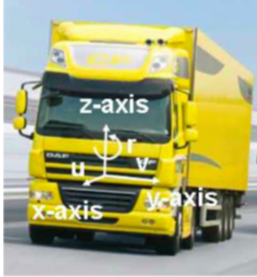
Figure 2-1: The body-fixed coordinates and forces affecting a vehicle. This figure is from [4]
