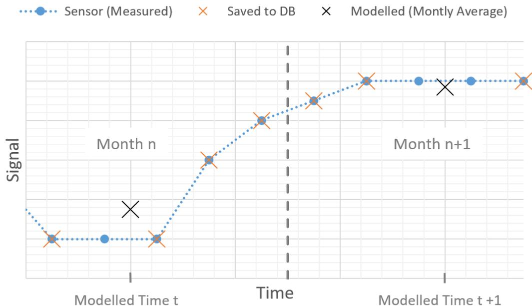
**Figure 23: Measured SCADA data, Saved Database Values and Modelled Values**
