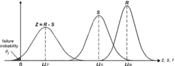
Figure 2. Distribution of potential values of loading f_S(s) and strength f_R(r) , plus the distribution of the limit state function f_Z(z) = f_R(r) - f_S(s) . A 'wide' distribution around the average limit state value \mu_Z implies a large uncertainty, while a 'tight' distribution indicates a high certainty. The failure probability P_f is represented by the area Z < 0 (the small black area left of the vertical axis). If the failure probability is lower than the acceptable target failure probability, the structure or system is considered sufficiently reliable.
