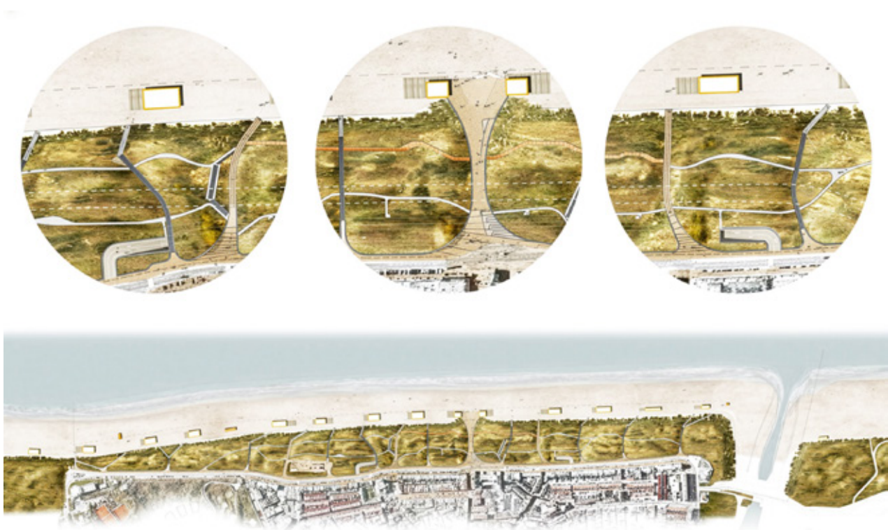
Spatial and engineering design of a dike and car park integrated in a dune landscape at the coastal zone Katwijk aan Zee. [© OKRA Landscape Architects]
