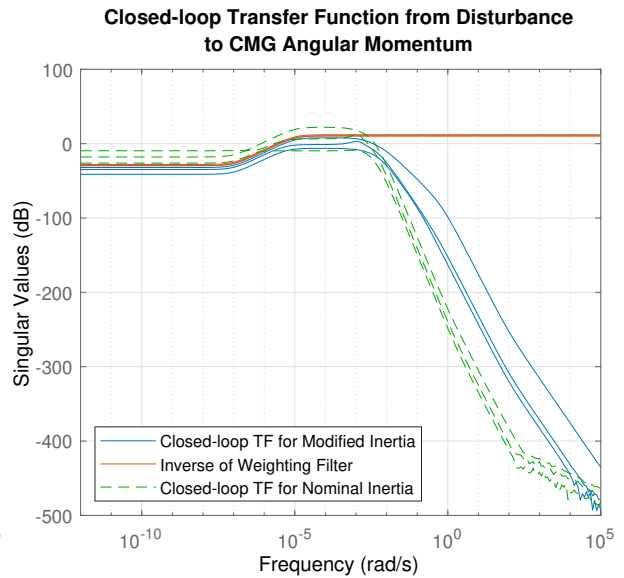
Fig. 14 Closed-loop transfer functions from disturbance to CMG angular momentum, considering the nominal and modified inertia
