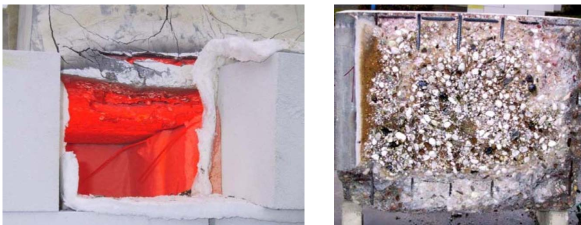
Fig. 2.22 Cracking of a slab during thermal exposure according to the RWS fire curve (left) and resulting spalling damage (right). The C85/100 concrete was made with quartz aggregates and stored under water before testing (Horvath, et al., 2004).
