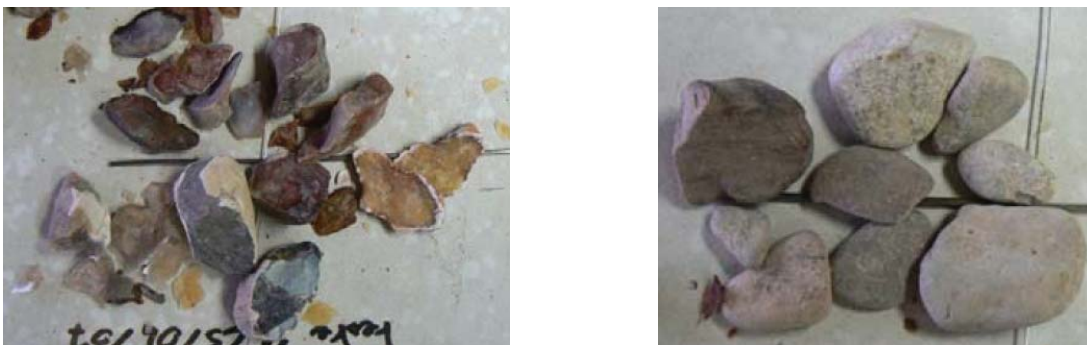
Fig. 2.4 Thermal instability of French flint (left), a siliceous aggregate type, compared to calcareous aggregates (right) after heating to a temperature of 200 °C (Mindeguia, 2009).
