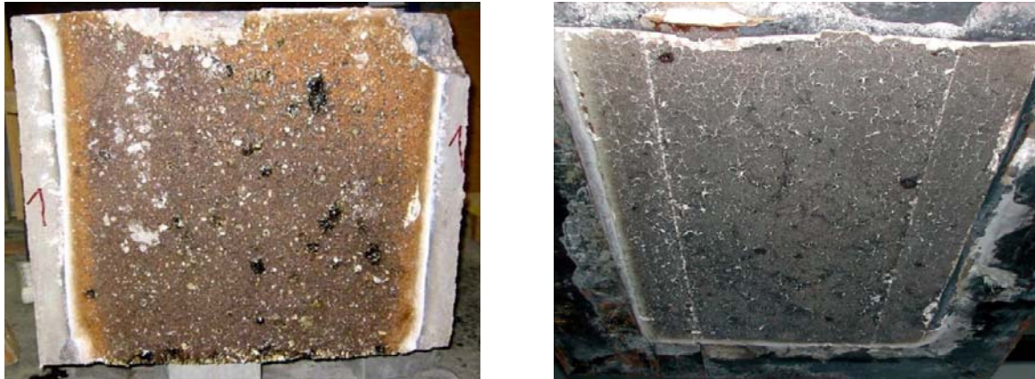
Fig. 2.26 Preventing spalling by addition of 2.0 \text{ kg/m}^3 of PP-fibres to the C85/100 mixture (left) (Horvath, et al., 2004). No damage occurred during testing of a compression loaded C25/30 slab made with 3.0 \text{ kg/m}^3 of PP-fibres (right) (FSV, 2004) Both slabs were stored under water before fire testing according to the RWS curve.
