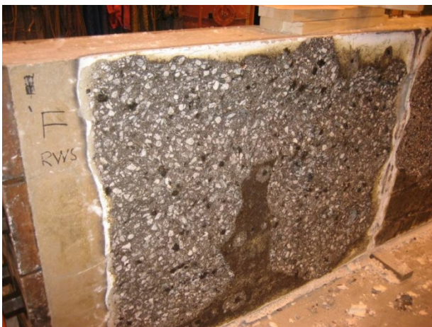
Fig. 1.10 Spalling of concrete can be limited to the surface as illustrated by the concrete slab after full-scale fire testing (left) (Jansson & Boström, 2008). The most severe spalling reduces the thickness and exposes the reinforcement as illustrated by the tunnel lining segment after the full-scale fire test (right) (picture taken at the MFPA 2 ).
