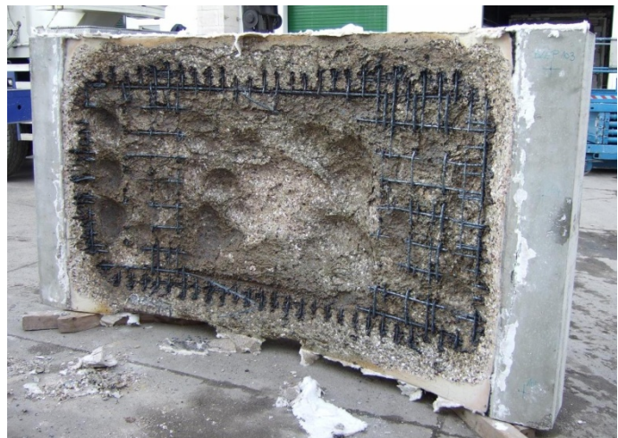
Fig. 1.10 Spalling of concrete can be limited to the surface as illustrated by the concrete slab after full-scale fire testing (left) (Jansson & Boström, 2008). The most severe spalling reduces the thickness and exposes the reinforcement as illustrated by the tunnel lining segment after the full-scale fire test (right) (picture taken at the MFPA 2 ).
