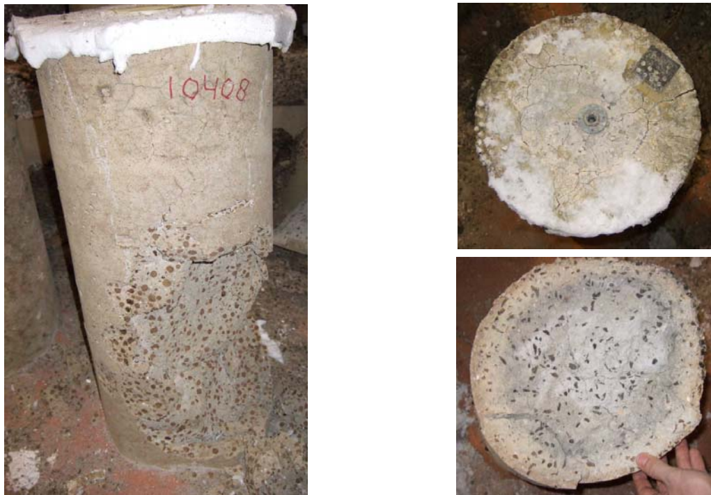
Fig. 2.18 Thermal expansion of the heated surface layer leading to a circular crack in the cross-section. In the centre a radial crack pattern developed (pictures taken at Efectis 6 ).
