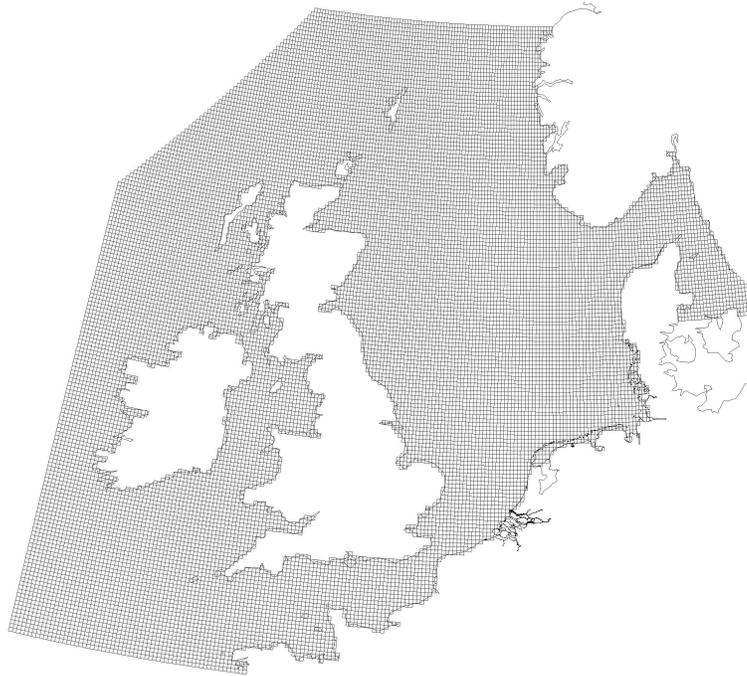
Figure 4.1: The grid of the Dutch Continental Shelf Model (DCSM). The DCSM model is a 2-dimensional model that is being used for day-to-day sea level forecasts.
