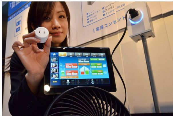
Figure 1.1: Sony’s Authentication Outlet employing RFID technology, [4].
